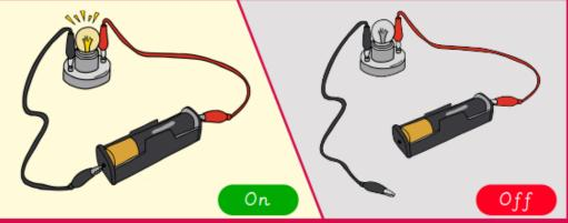
If there is a break in a series circuit, the electrical current will be cut and all the components will stop working. Causing a break in a series circuit can act as a switch to turn the circuit off.
