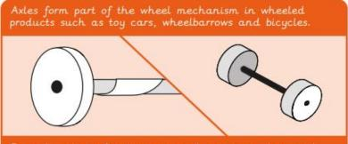
For a bicycle to function we need to use our legs and feet to push the pedals that rotate the axle and spin the wheels.
