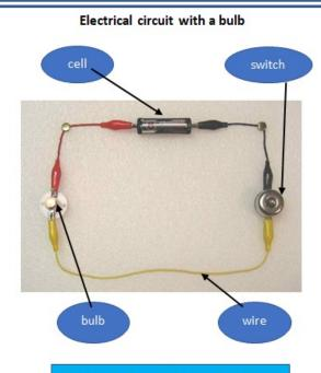
The switch opens and closes the circuit. The bulb lights in this circuit because the switch is on.
